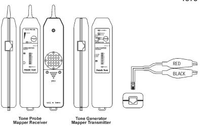
Tone Tracing Note: the tone signal only emits from the top RJ11 socket. Tone is NOT present on the side RJ45 socket
